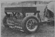
The new model has  $1\frac{1}{2}$  inch diameter spoons which penetrate to a maximum depth of six inches. The cultivating reel is made in two parts, the halves of the reel revolving independently on a fixed shaft to facilitate turning. There are eight rows of spoons staggered to make three holes per sq. ft. as it cultivates a swath  $5\frac{1}{2}$  feet wide or with three of the Aerifiers
