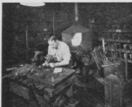
Bill Duncan, one of the skilled craftsmen who do the important work of making master models and special order irons, is checking a head with a precision gauge.
