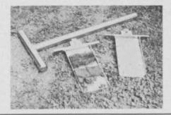
Take soil samples to find out the causes for poor turf and to check results of your improvement program. Take samples after watering greens to find out if water penetration has been adequate. The soil sample is seven inches deep. Cutting shell opens up so the soil is completely visible. The sample can be slipped back into place in the green after examination.
