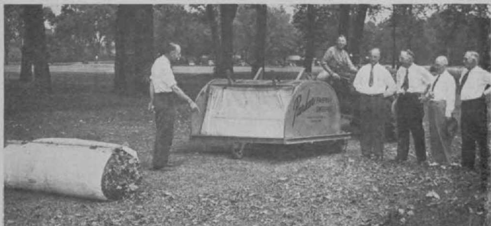
Russell Stout (left) designer of Parker Fairway Sweeper, explains to members of Snyder Park Golf Commission how machine collects leaves, twigs, golf balls, etc., and otherwise keeps fairways clean.
