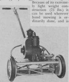
especially adaptable to cutting bunkers or steep terraces. The Sportlawn also has many of the features found on higher priced machines including finger-tip clutch and throttle controls, adjustable cutting height, semi-pneumatic tires, sectional rol-
