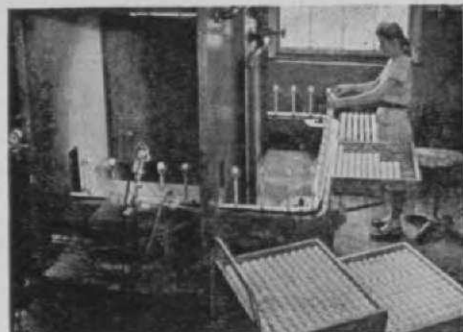
Automatic spraying machines are used for painting MacGregor golf balls. Flowing water in the interior of the spray booth removes all fumes and excess spray as operator feeds and removes painted balls while in same position.
