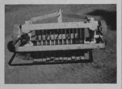
Illustration shows cultivating position. Weights on tray over axle regulate depth of cut. Circular knives made of fine knife steel. A real machine.
