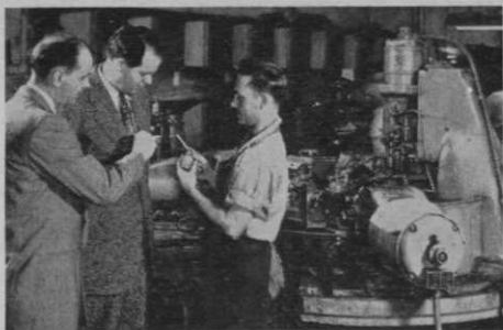
Ed Delahan, plant mgr., Golfcraft, Inc., and Ralph Guldahl inspect iron head with shaft hole in hozel bored and reamed to within .001 in. limit by special Kingsbury machine.
