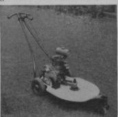
form construction permits mower to cut beneath hedges and shrubs without endangering their center trunks. It will cut a 24-in. swath with the greatest of ease. The blades can be sharpened merely by application to a grind stone or emery wheel.
