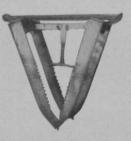
trigger trap springs the trap jaws. The trap is made of cold rolled steel. It is easy to see from quite a distance whether or not the trap has been sprung. Available from the makers, or golf course equipment dealers.
