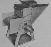
THIS MODEL comes in two sizes, feed opening 18 in. by 23 in. or 24 in. by 23 in. or 24 in. by 23 in. Other models to fit any compost grinding need. Cylinder assembly is built to stand shock of iron, rocks, and tramp material. Hammer bodies are ½ in. steel, 4 in. wide. Shaft is heavy alloy steel, mounted on heavy duty ball bearings. Designed for all types of power and for easy hookup. Patented features no other grinder has, make the W-W "the finest to be had."
