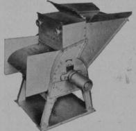
THIS MODEL comes in two sizes, feed opening 18 in. by 23 in. or 24 in. by 23 in. Other models to fit any compost grinding need. Cylinder assembly is built to stand shock of iron, rocks, and tramp material. Hammer bodies are ½ in. steel, 4 in. wide. Shaft is heavy alloy steel, mounted on heavy duty ball bearings. Designed for all types of power and for easy hookup. Patented features no other grinder has, make the W-W "the finest to be had."
