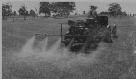
Sprayer in operation on rough. Boom on Hardie sprayer is home-made. Nozzles are cone-shaped type, spaced 18 inches apart, at 45 degree angle. The two end ones have separate shut-off and are on swivel so boom can be shortened. Upright mounting standards have holes 3 inches apart so height of boom from ground can be changed.
