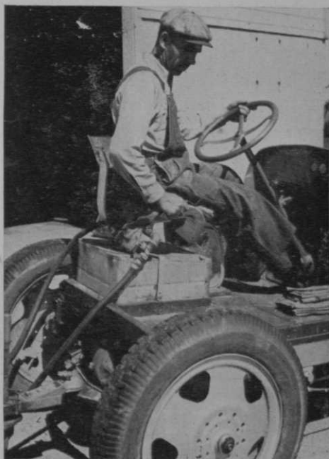
Hose from boom on the sprayer connects with shut-off valve on tractor.
