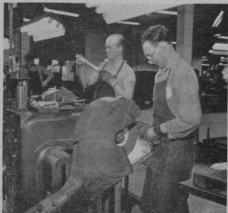
Workmen grind the final edge on bayonets at the American Fork plant.
