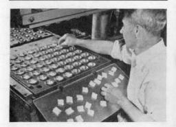
In "re-processing" used golf balls, according to the method announced by U. S. Rubber Co., the old covers will be removed and new covers will be moulded on the core. The new covers will be identical to the covers on new balls. Here the little white biscuits of Tjipetir, a special form of Balata, are placed on a cold press to be formed into shells. The shells will then be assembled on the winding and moulded in a hot press complete with dimples.
