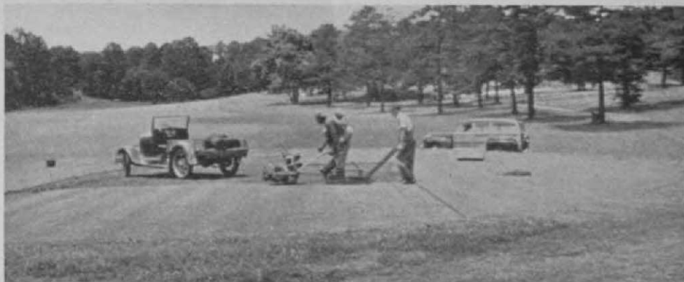
Another example of the wartime ingenuity of greenkeepers in cutting costs. A Toro Park Special is shown being used in cutting sod at the Biltmore Forest CC, Biltmore, N. C., where W. A. Bostic is supt.
