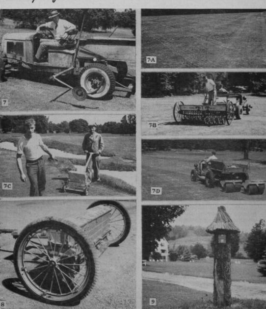
7—Improvised marker for spreader used to apply sodium arsenite by dry method, side view.
