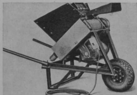
furnished with a 110/220 volt, single phase, 60 cycle, 1,750 R.P.M. motor. Mounted on a single
