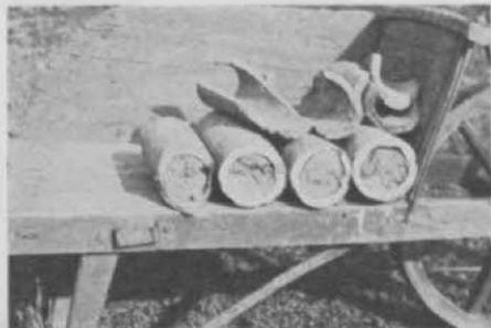
Samples of tile from a line that no longer drained. Do you wonder why?
