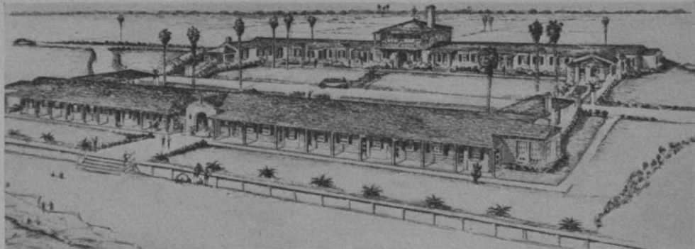
Now under construction as part of the $300,000 building program of the Ponte Vedra (Fla.) CC, hotel-resort of the Florida East coast, is this guest cottage section. It will consist of 33 guest rooms each 20 x 15 feet around a large central court. The section faces seaward to the Atlantic and landward to the main club building and golf links, and brings the accommodations at Ponte Vedra to 78 rooms.
