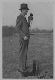
fits in coat pocket, and has a range between 1200 and 3600 feet, depending on conditions. Greater distance can be obtained with a small vacuum tube amplifier that I have designed. I have used this phone for distances up to 7200 ft.; remember pipe line distances are often greater than a bee-line.
