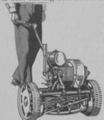
grip and wheels are automatically disconnected while cutting reel keeps whirling. Drop handle and both reel and wheels stop. Far-forward location of cutting bar
