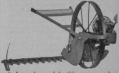
unit formerly used in this mower, when it was known as the Rawls motor scythe. This added power permits the sickle to saw through growths of weeds and brush that would stall a horse-drawn mower.
