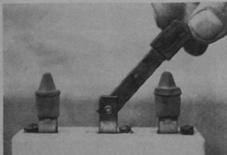
circuits when out of use during the winter. To prevent an accidental or ignorant closing of the switch, a neat little method is shown above.
