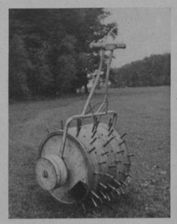
inch in diameter, so constructed to pierce the turf and at the same time cut a plug therefrom, leaving a clean-cut hole three inches deep in the turf.
