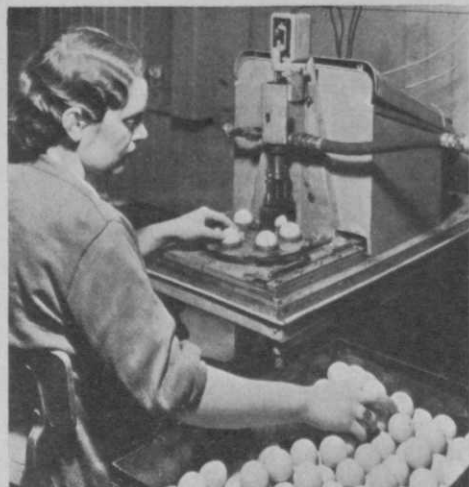
This machine needles the Krollite cores.
