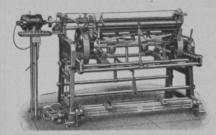
blade so that both the face and the edge can be ground quickly and accurately in one setting by rotating the bar.
