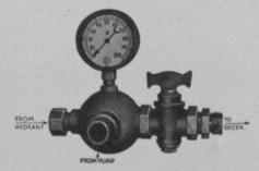
with fungicides, fertilizers, etc. It is attached to a barrel pump, the hydrant and the hose leading to the green, as indicated in the cut. Chemical solutions are pumped
