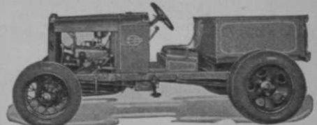
Steel tractor wheels interchangeable with Ford pneumatic-tired wheels for paved roads.
