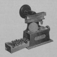
ball against the straight face of the type, according to the makers, produces a clear, perfect marking and does not injure even the thinnest balata covers of the finest hard-wound, long-distance balls.
