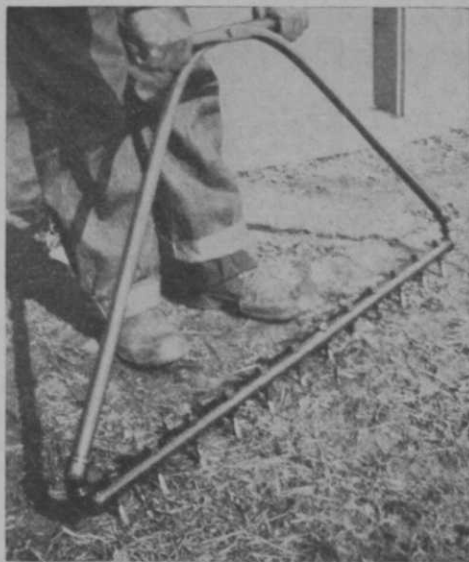
Close-packed soil responds quickly to the leverage action possible with this aerator.
