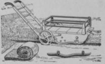
A PROFITABLE time and labor saver that gives a neater job of sodding. Cuts a strip 14 inches wide; adjustable, uniform thickness; any length desired. Makes a smoother, firmer turf especially on embankments. Made for either horse power or tractor.
