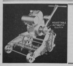
A Hand Propelled power operated double reel machine for renovating, cultivating, disking and conditioning
