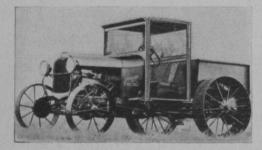
it can be attached quickly and easily to any Model "A" Staude tractor.
