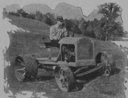
The chassis on the new Toro Junior is built of four-inch steel channel sections, and will remain absolutely rigid, regardless of operating difficulties.
