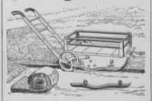
A PROFITABLE time and labor saver that gives a neater job of sodding. Cuts a strip 14 inches wide; adjustable, uniform thickness; any length desired. Makes a smoother, firmer turf especially on embankments. Made for either horse power or tractor.
