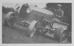
Electric starter, battery, lights, shock absorbers, a silent (enclosed in oil) worm gear truck drive differential.
