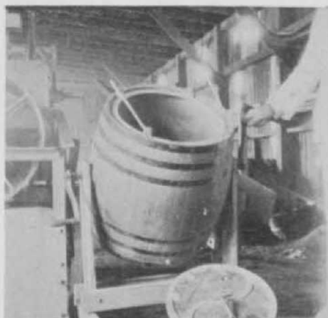
This churn mixed the compost efficiently and rapidly.
