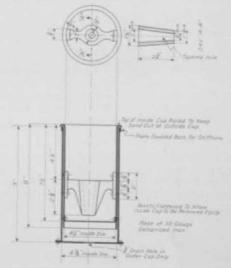
sleeves by four knurls or round-headed rivets ground on one side so that there are shoulders to hold the regulation cup from dropping down. Then we use a prepared auger arrangement for lifting the sand out of the cups about once a week.
