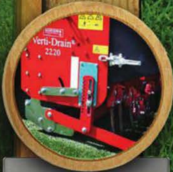
Depth adjustments made from the tractor seat
