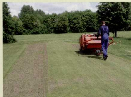
CORE RECYCLER Re-use sand, collect thatch.
