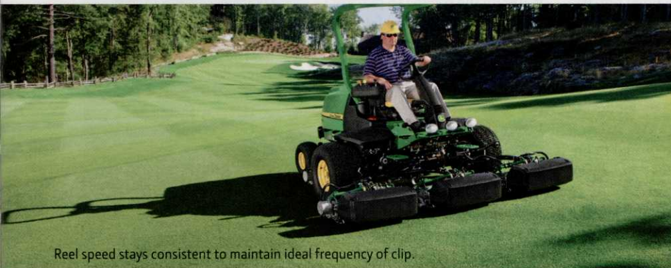
Electric reel motors require no routine service.
