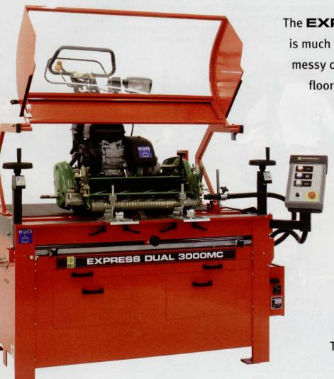
The **EXPRESS DUAL** spin grinder is much faster than back-lapping with no messy cleanup. Fifteen minutes floor-to-floor for a reel grind makes lapping a thing of the past.
