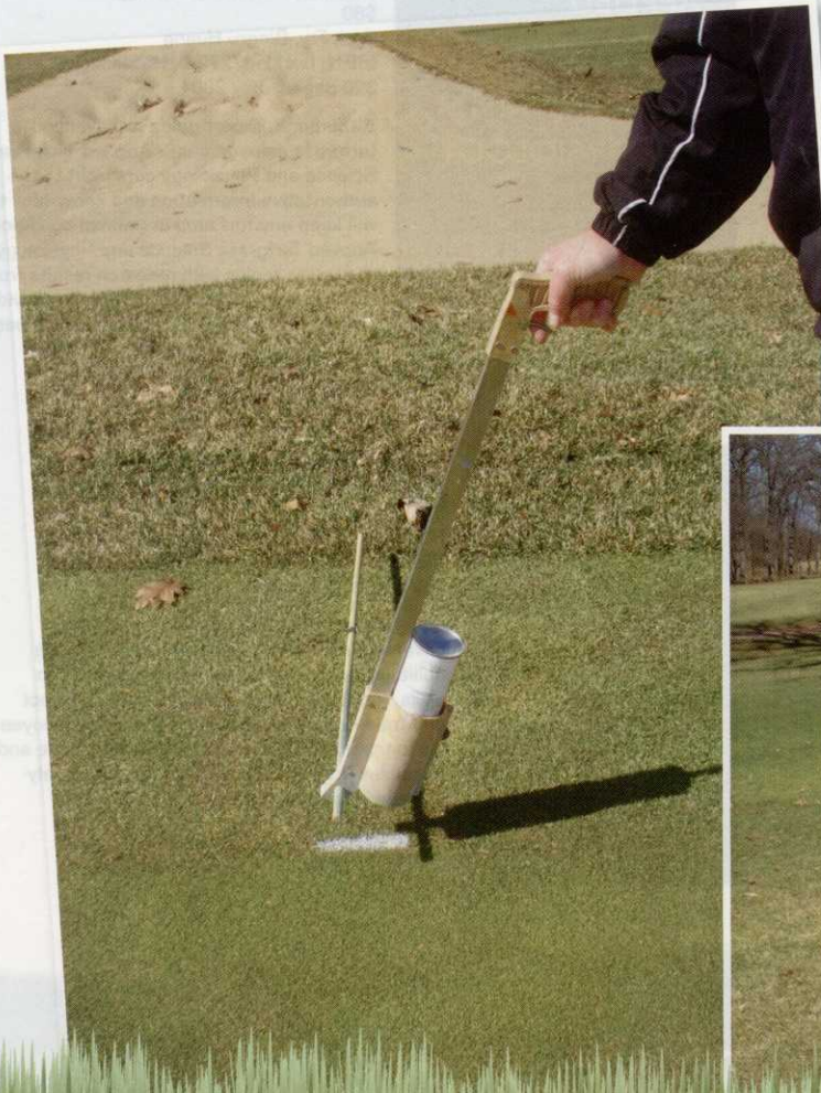
To keep greens from shrinking, Dave Schlagetter, GCCS at Indian Hill Club in Winnetka, Ill., uses a spray gun with 36-inch dowel rod attached to mark points to indicate where mower operators' edges should be.
