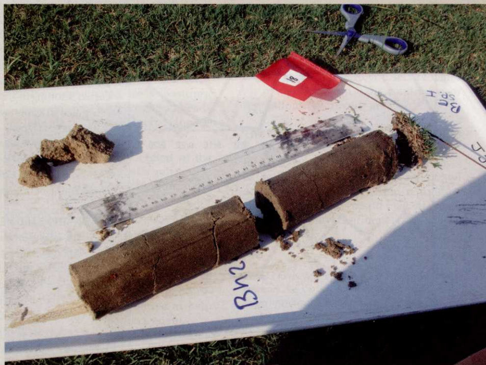
Cores were collected before and after the experiment to determine if irrigating with saline water influenced stolon density and root mass.
