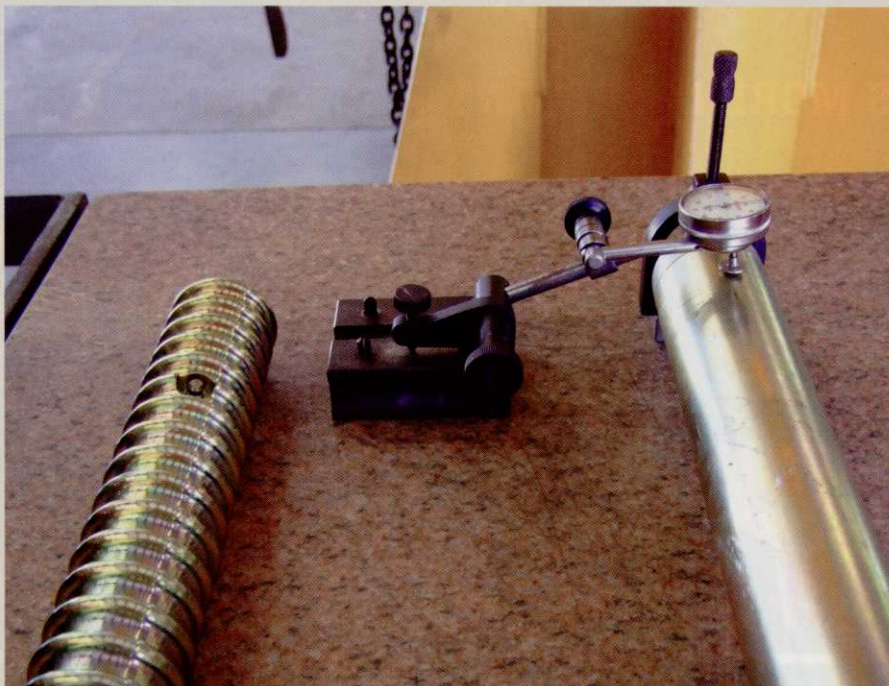
Gauge blocks and a dial indicator are used to measure runout by spinning a roller and recording the amount of difference on both ends. Photo: Stephen Tucker
