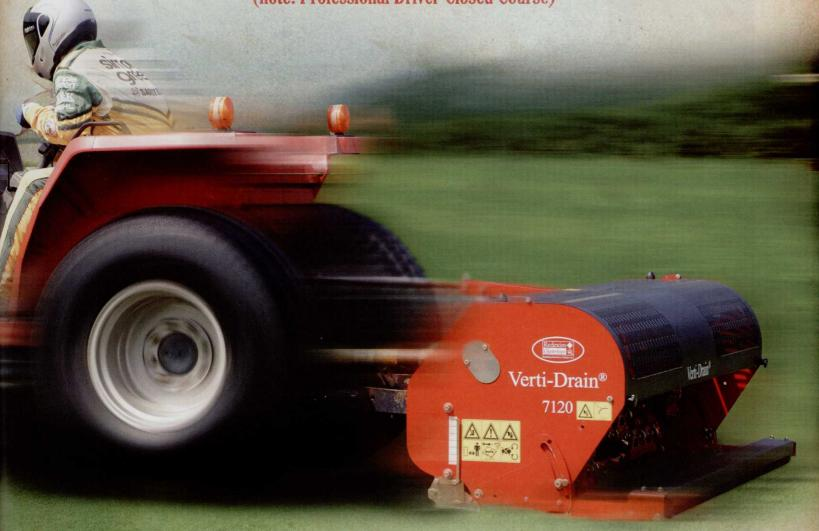
The new Verti-Drain 7120 outperforms all challengers as the fastest aerator on the course. At depths up to 8 inches and speeds over 3 MPH, the 7120 can aerate hard compacted soil fast and easy. With an 80 inch working width to maximize operating efficiency, the Verti-Drain 7120 is aimed at professionals that are not afraid to go fast.
