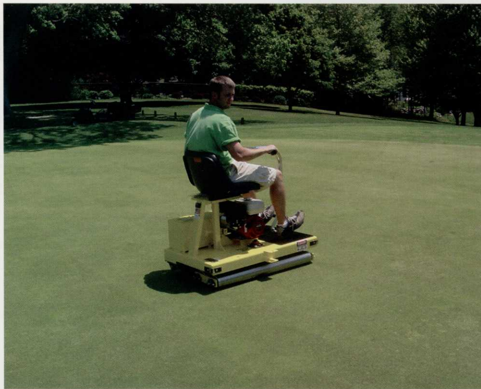
It's possible to raise the height of cut on greens 25 percent by rolling them, says John Fulling, CGCS. Photo: Kalamazoo Country Club
