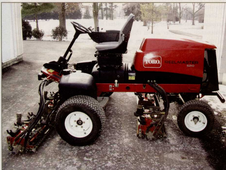
Because the fairways at Ulen Country Club were converted from ryegrass to bentgrass, Jeff Mann needed to increase the number of blades per reel on fairway units. Photo: Jeff Mann
