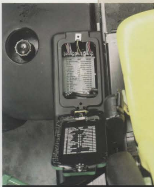
John Deere's White Box determines where power interruption occurs. Photo: John Deere
