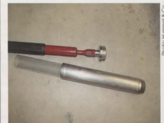
Special equipment can be used to pull undisturbed soil samples from greens.
